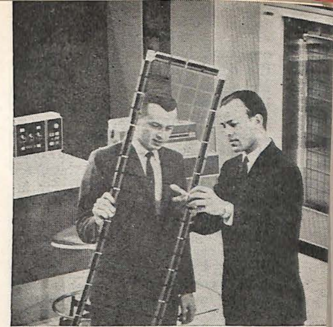
The core storage memory system of the IBM-360. Arrays of these core planes, resembling small screen doors, can be linked to put each of 8,000,000 or more characters at the direct command of the computer programmer in eight-millionths of a second.
