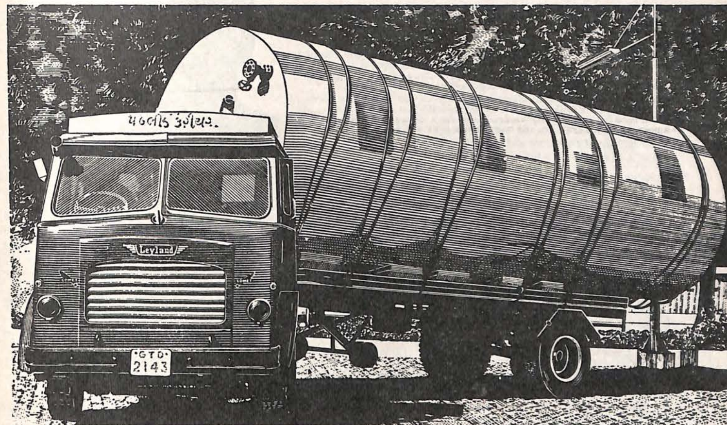
Ashok Leyland Comet tractor-trailer coupled with Mahindra Owen "Gama" semi-trailer hauling a 11-ton boiler 25'4" long and 9' high
